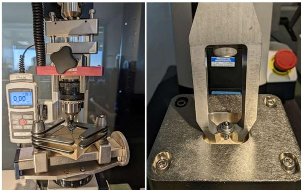
Figure 2: Screw insertion with Mark-10 TSTM-DC-1 (left) and screw pullout with Mark-10 ESM303 (right).
