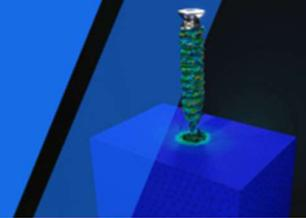
density can result in more than 10% difference in terms of maximum pullout force (Weidling, Wendler, et al., 2022). This discrepancy may even surpass the impact of certain screw features, which complicates the design assessment process. Although increasing the number of repetitions can improve the statistical reliability of results, it also extends the duration of testing, which can be time-consuming and costly.
