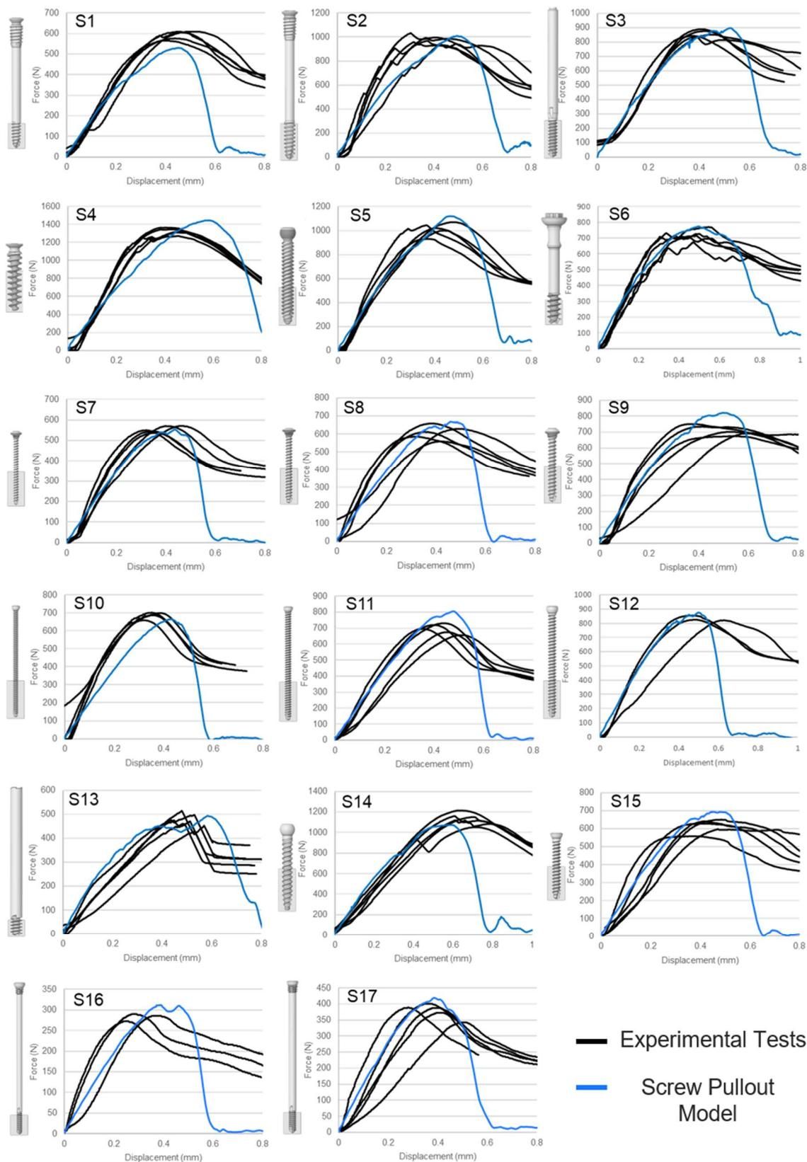
Figure 4: Experimental (black) and simulated (blue) screw pullout force-displacement curves.
